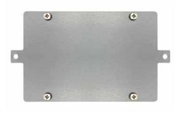
**Step 4** Lock up HDD bracket on HDD cover with 2 pcs screws.
